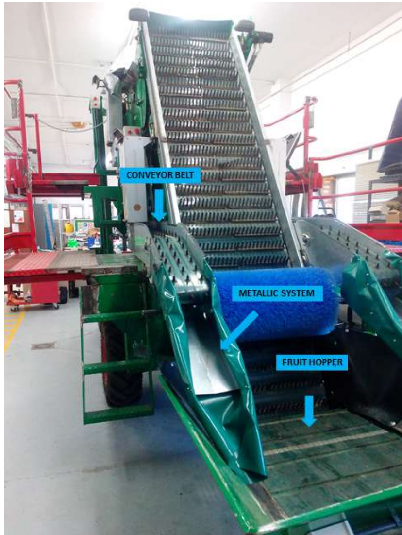
Figure 4. Conveyor belt and metallic system placed before the fruit hopper in the prototype.
