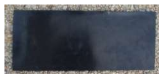
Material 7 Density: 146.87 \text{ Kg m}^{-3} Thickness: 3.10 mm Figure 3. Materials.
