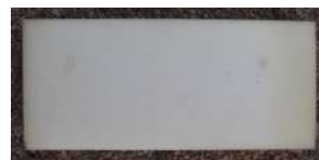
Material 2 Density: 26.74 \text{ Kg m}^{-3} Thickness: 43 mm
