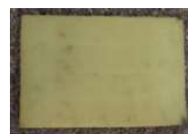
Material 6 Density: 18.26 \text{ Kg m}^{-3} Thickness: 18 mm
