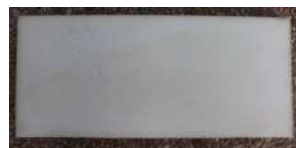
Material 1 Density: 46.36 \text{ Kg m}^{-3} Thickness: 41 mm
