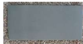
Material 4 Density: 23.37 \text{ Kg m}^{-3} Thickness: 10 mm
