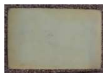
Material 5 Density: 16.44 \text{ Kg m}^{-3} Thickness: 9 mm
