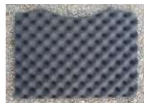
Material 3 Density: 15.56 \text{ Kg m}^{-3} Thickness: 23.25 mm
