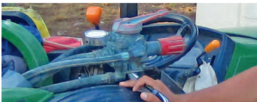
Fig. 8. High-pressure conduits in the tractor cabin.
