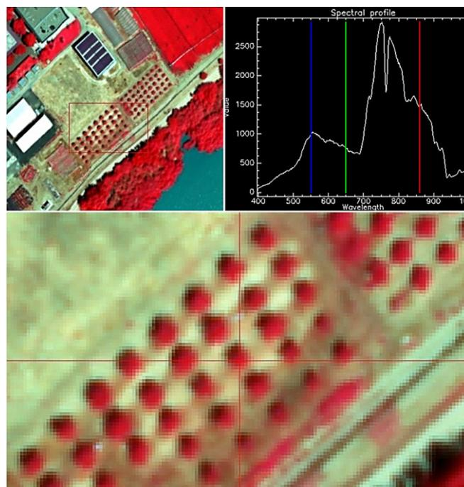
**Fig. 2** Hyperspectral image acquired from an airborne platform. The spectral profile extracted from each pixel and from entire tree crowns (top right) are used for the calculation of stress indicators related to tree physiological status and disease severity levels. Courtesy of the Laboratory for Research Methods in Quantitative Remote Sensing (QuantaLab), IAS-CSIC, Cordoba, Spain, <http://quantalab.ias.csic.es>.
