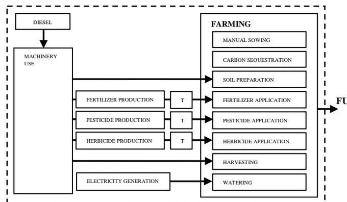
Figure 2. Substages included in the system under study for the cradle-to-farm gate LCA.
