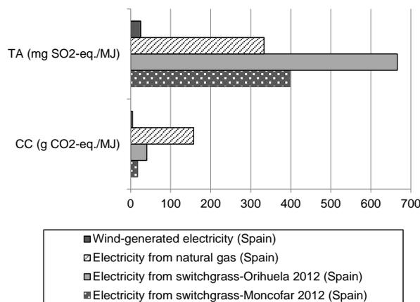
Figure 4. Climate change (CC) and terrestrial acidification (TA) emission factors, in terms of g of CO<sub>2</sub>-eq. MJ<sup>-1</sup> and mg of SO<sub>2</sub>-eq. MJ<sup>-1</sup>, respectively, for four options for electricity production in Spain.
