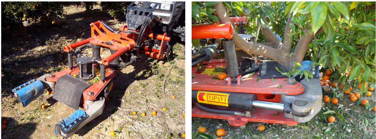
Figure 1. Trunk shaker used during the experiments. Left: trunk shaker with the shaker clamps open. Right: shaker attaching the mandarin trunk.
